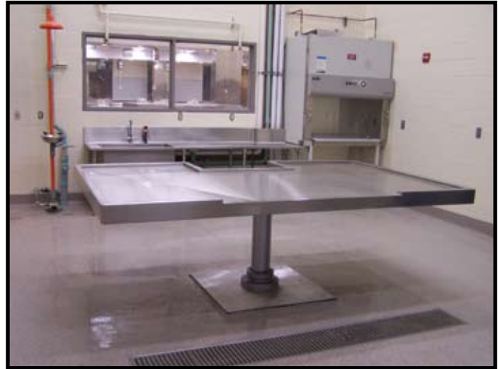
EXPOSED PISTON SHOWN RECESSED INTO THE GROUND
