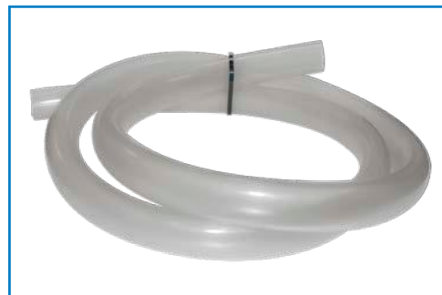
AHS - ASPIRATOR DISCHARGE TUBING 3 ft. min., priced per foot. Splash tubing for aspirator drain, embalming and autopsy tops. Internal diameter of 1 in. and outside diameter of 1.25 in..
