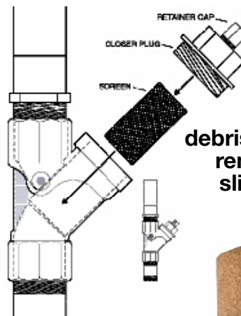
WYE STRAINER PLUMBED INTO A 1036-10
