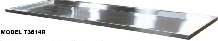
A real time and energy saver, the detachable stainless steel top will ensure a secure fit with no mechanical fastening devices required. It is fabricated from 14 gauge 304 stainless steel with No. 4 finish. Interior long sides are angled to allow for easier body transfer. It features a depressed pattern allowing fluids to drain easily.
