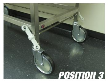
POSITION 3: Back Tilt, Brake . All casters are locked from rotation and forward and backward movement. Use this when loading or unloading body into position to ensure safety and avoid injury.
