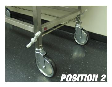
POSITION 2: Forward Tilt, Steer. Casters are partially locked into position except, for the front left caster (opposite the controls). Used for better steering and control when operating the carrier.
