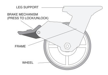
Pull upward or push upward on the top of the locking mechanism to release
