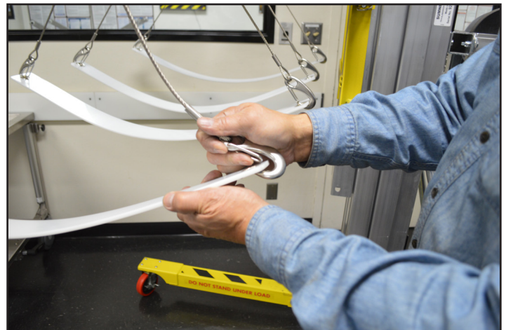
2. Secure Glide Straps with the D-Ring w/Snaps.
