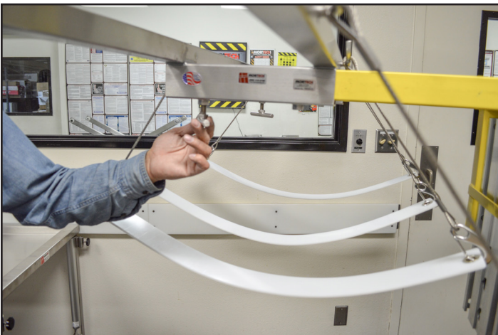
1. Turn the Locking Bolt to secure the M605
