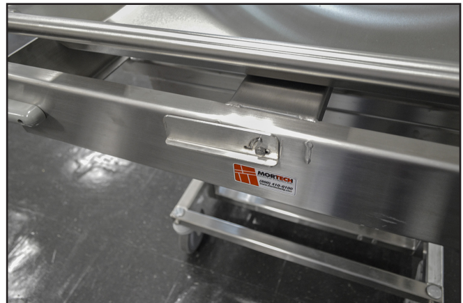
Flip tray latches downward to allow free movement of tray
