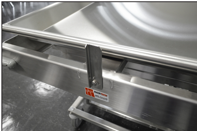
Flip tray latches up to restrict free movement of tray
